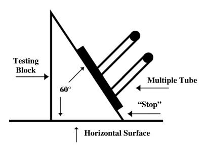
Side view of an apparatus or testing block for testing compliance with the 60-degree tilt angle standard.
